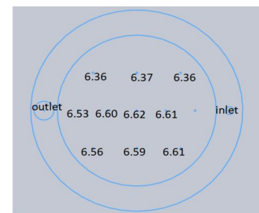
Fig. 3 the thickness of aluminum oxide ( 6.52 \pm 0.11 nm)
